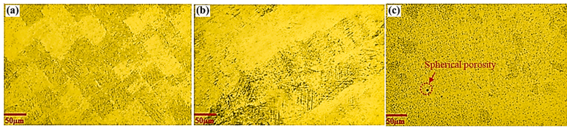
Fig. 3. The OM images of the (a) SLM-XY, (b) SLM-XX, and (c) EBM XX samples.
