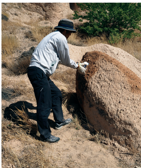
Fig. 1 — Dr. Katsuhiko Sano applying an alkoxy-silane-based coating on a rock surface in Cappadocia, Turkey. Courtesy of D&D K.K.
