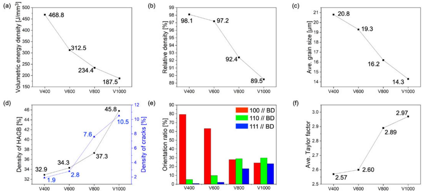
**Figure 4.** Plots of (a) volumetric energy density, (b) relative density, (c) average grain size, (d) density of HAGB and crack density, (e) orientation ratio, and (f) average Taylor factor from V400, V600, V800, and V1000 samples.
