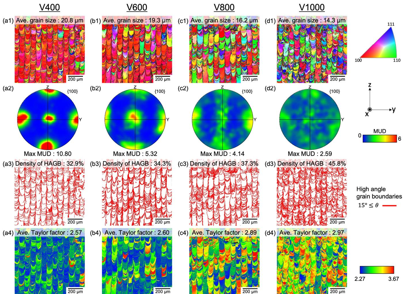
**Figure 3.** (a1–d1) IPF maps along BD and (a2–d2) {100} pole figures of the y-z plane orientation in the Z-direction. (a3–d3) Corresponding high-angle grain boundary maps and (a4–d4) Taylor factor maps.
