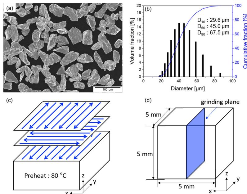
**Figure 1.** (a) Morphology and (b) particle size distribution of pure Cr powders, (c) schematic representation of the laser scan strategy; blue arrows mean laser scan path, and (d) schematic representation of the sample preparation for the observation.
